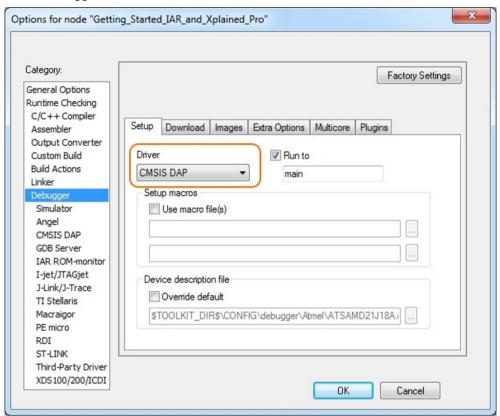
Figure 5-3. Configure Flash Loader
