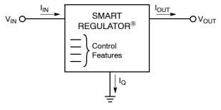
Figure 14. Single Output Regulator With Key Performance Parameters Labeled
