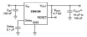
\*C<sub>IN</sub> is required if regulator is far from the power source filter. \*\*C<sub>OUT</sub> is required for stability.
