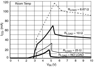
Figure 3. Quiescent Current vs. Input Voltage Over Load Resistance
