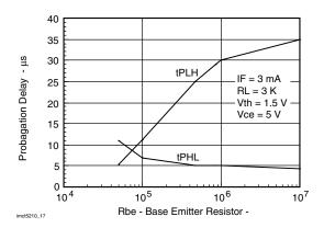
Fig. 17 - Propagation Delay vs. Base Emitter Resistor
