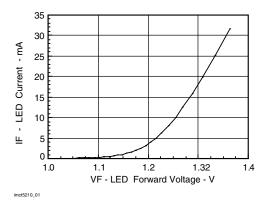
Fig. 3 - Forward Current vs. Forward Voltage
