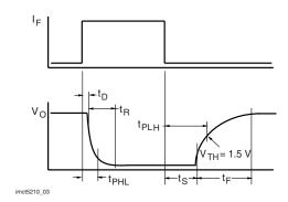
Fig. 2 - Switching Waveform
