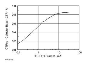
Fig. 8 - Collector Base CTR vs. LED Current
