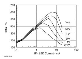
Fig. 9 - CTR vs. LED Current
