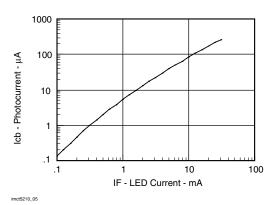
Fig. 6 - Photocurrent vs. LED Current
