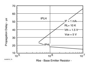
Fig. 15 - Propagation Delay vs. Base Emitter Resistor
