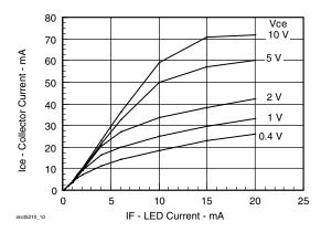
Fig. 10 - Collector Current vs. LED Current
