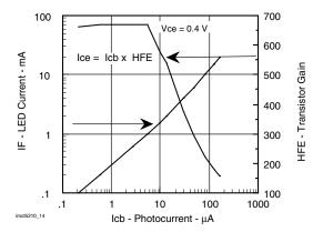
Fig. 14 - Transfer Curve
