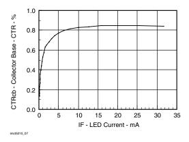
Fig. 7 - Collector Base CTR vs. LED Current
