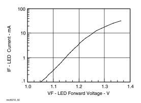
Fig. 4 - LED Forward Current vs. Forward Voltage
