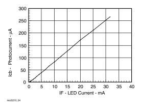
Fig. 5 - Collector Base Photocurrent vs. LED Current
