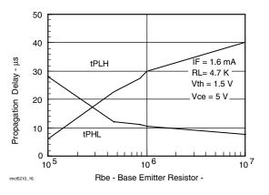
Fig. 16 - Propagation Delay vs. Base Emitter Resistor
