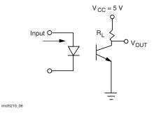
Fig. 1 - Switching Schematic
