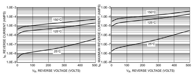
**Figure 3. Typical Reverse Current**
