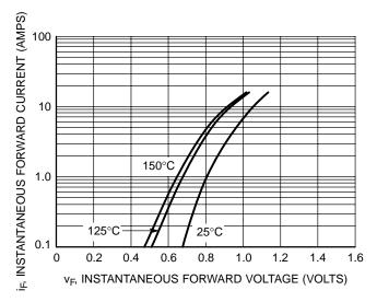
Figure 1. Typical Forward Voltage
