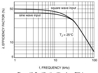
Figure 10. Rectification Waveform Efficiency
