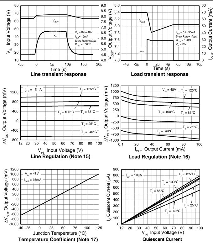
Notes: 15. Line regulation  $\Delta V_{OUT} = V_{OUT} - V_{OUT}$  (@  $V_{IN} = 12V$ ,  $I_{OUT} = 15mA$ ,  $T_J = +25^{\circ}C$ )
