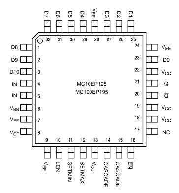
Figure 1. 32-Lead LQFP Pinout (Top View)
