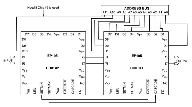
Figure 6. Cascading Interconnect Architecture
