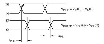
Figure 5. AC Reference Measurement
