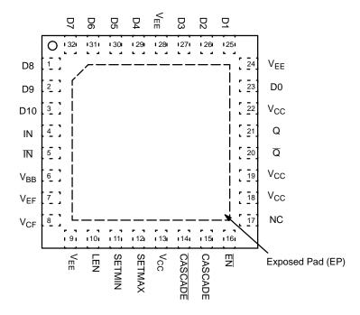
Figure 2. 32-Lead QFN (Top View)
