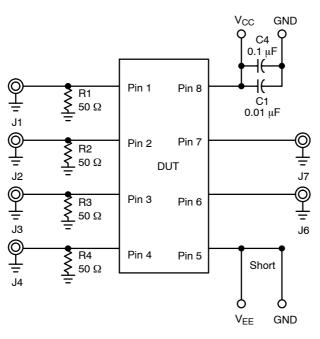
Figure 12. Configuration 9 – Translator Schematic (Unloaded Testing Condition)
