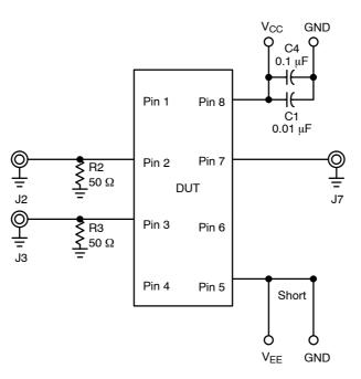
Figure 10. Configuration 7 – Translator Schematic (Unloaded Testing Condition)
