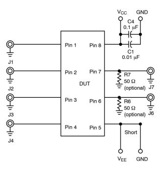
Figure 11. Configuration 8 – Translator Schematic
