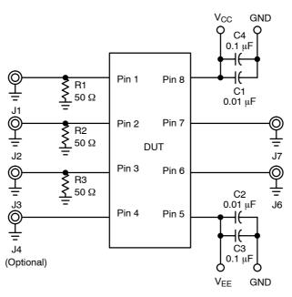
Figure 7. Configuration 4 Schematic
