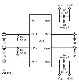
Figure 5. Configuration 2 Schematic
