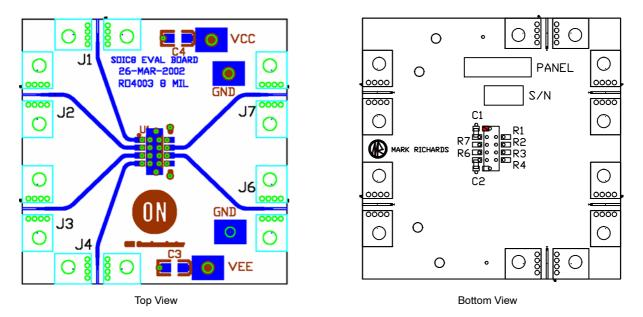
Figure 3. Evaluation Board Layout
