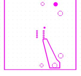
Second Layer (V<sub>EE</sub> and Ground Plane
