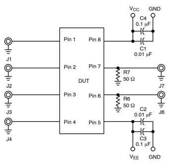
Figure 6. Configuration 3 Schematic
