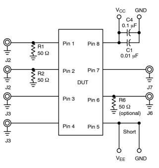
Figure 14. Configuration 11 – Translator Schematic
