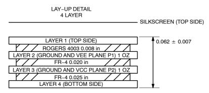
Figure 2. Evaluation Board Lay-up
