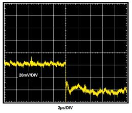
Figure 12. Typical Transient Response for Design Example Load Step
