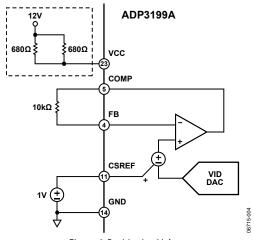
Figure 6. Positioning Voltage
