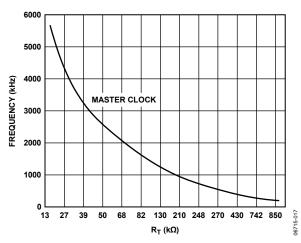
Figure 3. Master Clock Frequency vs. R<sub>™</sub>
