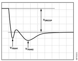
Figure 16. Transient Setting Waveform
