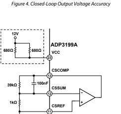
Figure 5. Current Sense Amplifier Offset Voltage (Vos)
