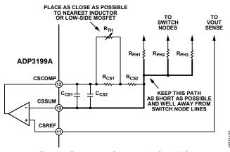
Figure 11. Temperature-Compensation Circuit Values
