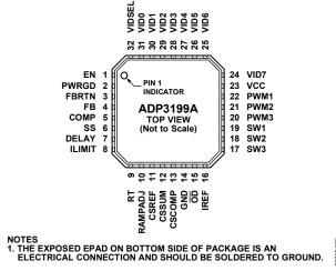
Figure 2. Pin Configuration
