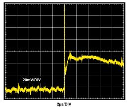
Figure 13. Typical Transient Response for Design Example Load Release
