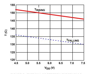
FIGURE 5. THERMAL PROTECTION THRESHOLDS
