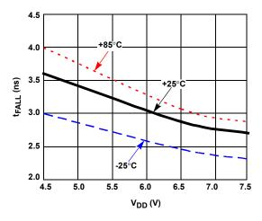
FIGURE 17.  $t_{FL}$  WITH TEMPERATURE ( $C_{GL} = 3nF$ , LSEL = VDD)
