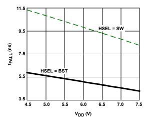
FIGURE 24. HIGH-SIDE DRIVER FALL TIME, t<sub>FH</sub> (CGH = 3nF,  $T_{\Delta} = +25^{\circ}C$
