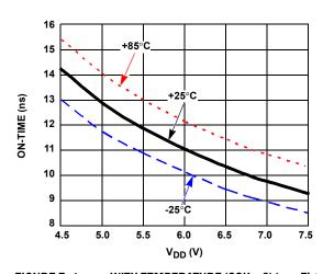
FIGURE 7.  $t_{GH,ON}$  WITH TEMPERATURE (CGH = 0) (see Figure 3 for  $t_{GH,ON}$  timing)
