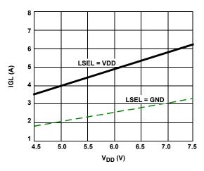
FIGURE 12. LOW-SIDE DRIVER PULL-DOWN CURRENT ( $V_{GL}$  = 2.5V,  $T_A$  = +25 °C)
