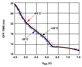
FIGURE 9. MINIMUM PWMH OFF-TIME,  $t_{PWMH,OFF}$  (CGH = 0)
