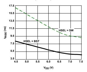
FIGURE 22. HIGH-SIDE DRIVER RISE TIME, t<sub>RH</sub> (CGH = 3nF,  $T_{\Delta} = +25^{\circ}C$
