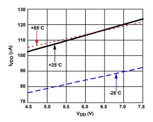
FIGURE 4. I<sub>VDD</sub> vs V<sub>DD</sub> WITH TEMPERATURE (NO SWITCHING)
