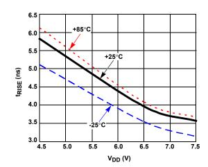
FIGURE 15. t<sub>RL</sub> WITH TEMPERATURE (C<sub>GL</sub> = 3nF, LSEL = VDD)
