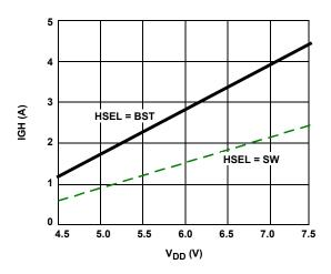
FIGURE 18. HIGH-SIDE DRIVER PULL-UP CURRENT ( $V_{GH}$  -  $V_{SW}$  = 2.5V,  $T_A$  = +25°C)
