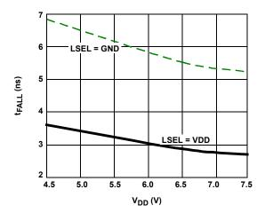
FIGURE 16. LOW-SIDE DRIVER FALL TIME,  $t_{FL}$  (CGL = 3nF,  $T_A$  = +25 °C)
