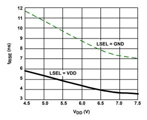
FIGURE 14. LOW-SIDE DRIVER RISE TIME,  $t_{RL}$  (CGL = 3nF,  $T_A$  = +25 °C)
