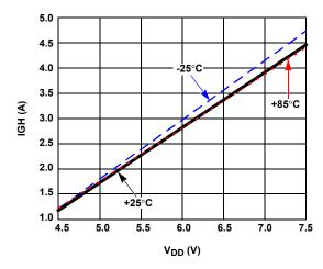
FIGURE 19. HS PULL-UP CURRENT WITH TEMPERATURE (V $_{\rm GH}$  - V $_{\rm SW}$  = 2.5V, HSEL = BST)
