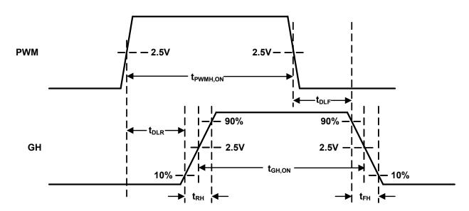
FIGURE 3. TIMING DIAGRAM
