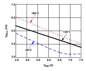
FIGURE 25. t<sub>FH</sub> WITH TEMPERATURE (C<sub>GH</sub> = 3nF, HSEL = BST)
