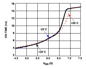
FIGURE 8. MINIMUM PWMH ON-TIME,  $t_{PWMH,ON}$  (CGH = 0)
