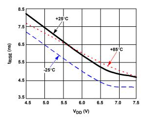
FIGURE 23. t<sub>RH</sub> WITH TEMPERATURE (C<sub>GH</sub> = 3nF, HSEL = BST)
