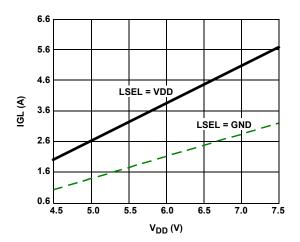
FIGURE 10. LOW-SIDE DRIVER PULL-UP CURRENT ( $V_{GL} = 2.5V$ ,  $T_A = +25$  °C)
