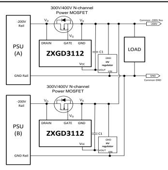
The focus application of the ZXGD3112 OR-ing Controller is for Redundant Low-Side -200V Power Supply Rail. HV to 12V regulator or a potential divider is suggested to power the  $V_{CC}$  of ZXGD3112 from high voltage lines.
