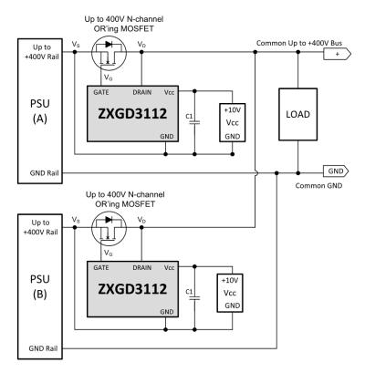
Example of the ZXGD3112 OR-ing Controller in a Redundant High-Side +200V Power Supply Rail using an additional V<sub>CC</sub> supply.
