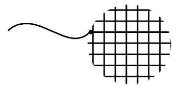
show that the electrode has more capacitance than the QT110 can tolerate, the electrode can be made into a sparse mesh (Figure 1-4) having lower Cx than a solid plane. Sensitivity may even remain the same, as the sensor will be operating in a lower region of the gain curves.
