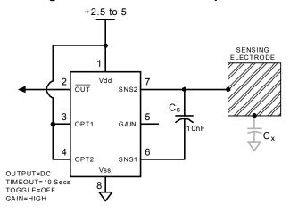
The IC is highly tolerant of changes in Cs since it computes the threshold level ratiometrically with respect to absolute load, and does so dynamically at all times.
