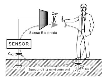
Figure 1-6 Shielding Against Fringe Fields
