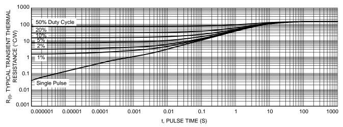
Figure 8. Typical Transient Thermal Response, Junction-to-Ambient
