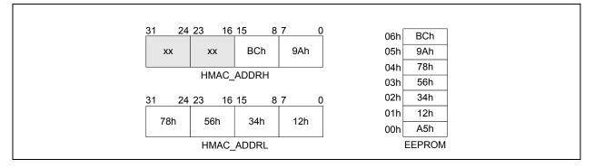
**Note:** By convention, the right nibble of the left most byte of the Ethernet address (in this example, the 2 of the 12h) is the most significant nibble and is transmitted/received first.
