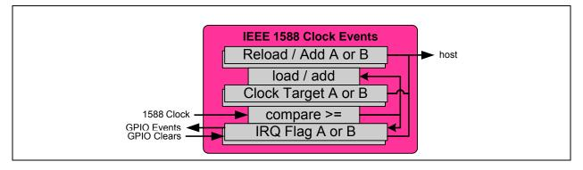
For each clock event channel, a comparator compares the 1588 Clock with a Clock Target loaded in the 1588 Clock Target x Seconds Register (1588\_CLOCK\_TARGET\_SEC\_x) and 1588 Clock Target x NanoSeconds Register (1588\_CLOCK\_TARGET\_NS\_x).
