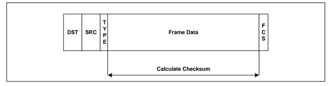
In mode 1, the RXCOE supports VLAN tags and a SNAP header. In this mode, the RXCOE calculates the checksum at the start of L3 packet. The VLAN1 tag register is used by the RXCOE to indicate what protocol type is to be used to indicate the existence of a VLAN tag. This value is typically 8100h.
