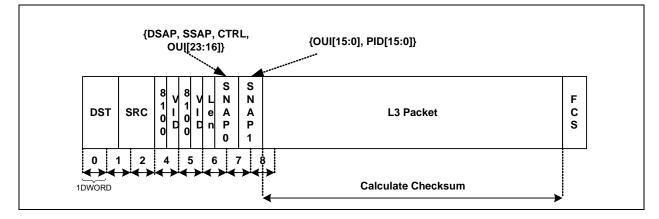
The RXCOE supports a maximum of two VLAN tags. If there are more than two VLAN tags, the VLAN protocol identifier for the third tag is treated as an Ethernet type field. The checksum calculation will begin immediately after the type field.
