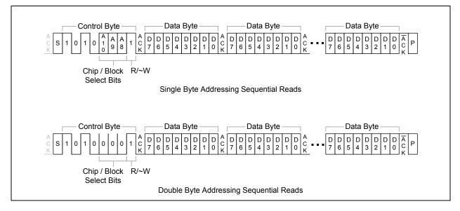
Sequential reads are used by the EEPROM Loader. Refer to Section 13.4, "EEPROM Loader" for additional information. For a register level description of a read operation, refer to Section 13.3.7, "I2C Master EEPROM Controller Operation,"
