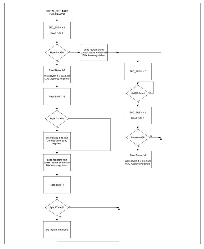
FIGURE 13-8: EEPROM LOADER FLOW DIAGRAM
