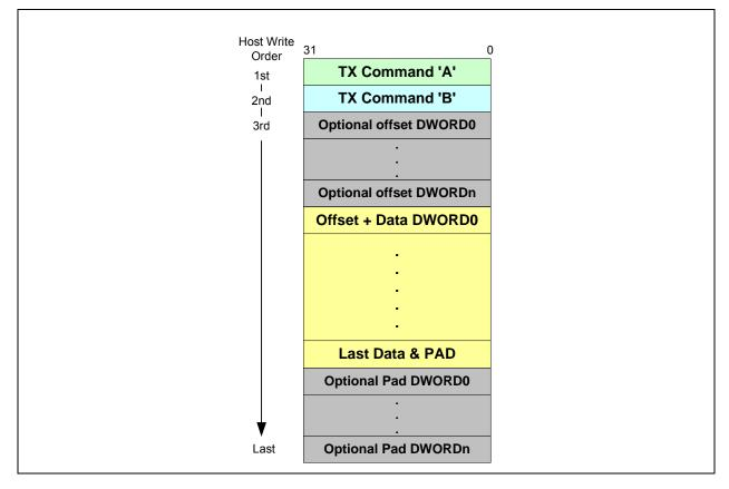
FIGURE 11-11: TX BUFFER FORMAT
