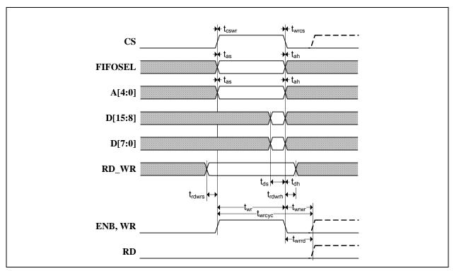
FIGURE 9-44: INDEXED ADDRESSING WRITE CYCLE TIMING
