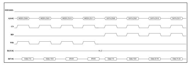
FIGURE 9-32: INDEXED ADDRESSING INTERNAL REGISTER DATA ACCESS - 8-BIT READ
