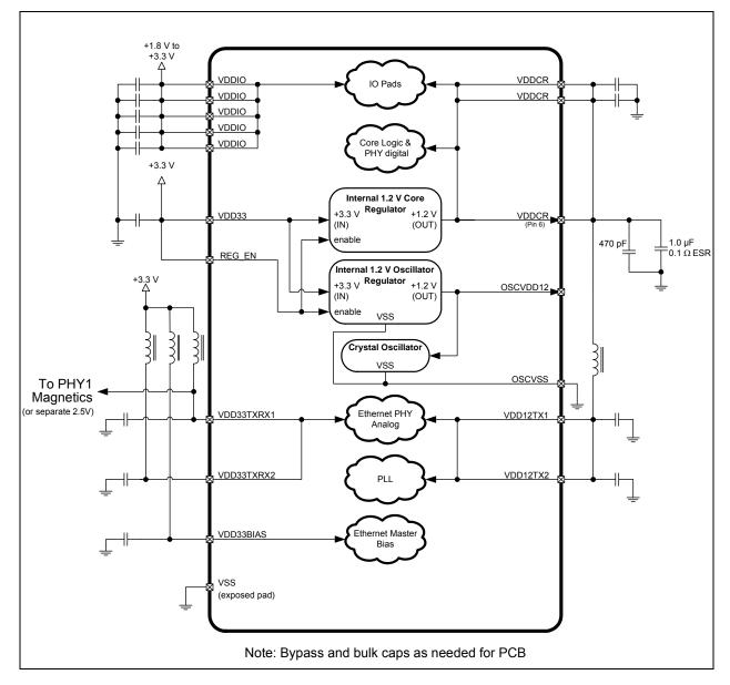
FIGURE 4-1: POWER CONNECTIONS - REGULATORS ENABLED
