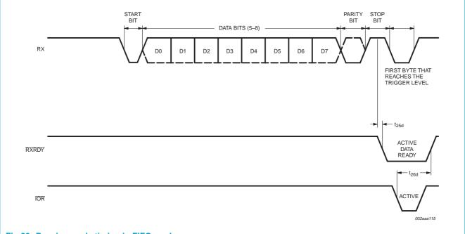
Fig 20. Receive ready timing in FIFO mode.
