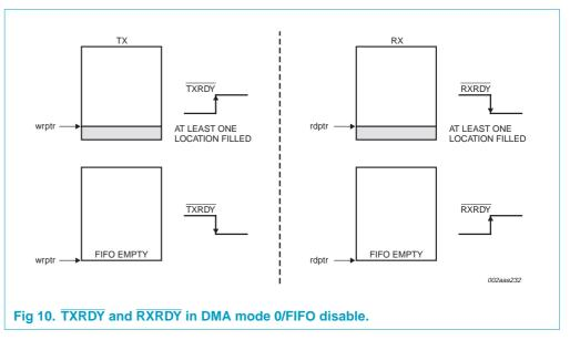
**Transmitter:** When empty, the TXRDY signal becomes active. TXRDY will go inactive after one character has been loaded into it.
