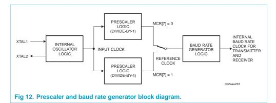
DLL and DLH must be written to in order to program the baud rate. DLL and DLH are the least significant and most significant byte of the baud rate divisor. If DLL and DLH are both zero, the UART is effectively disabled, as no baud clock will be generated.
