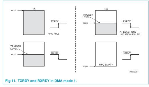
**Transmitter:** TXRDY is active when there is a trigger level number of spaces available. It becomes inactive when the FIFO is full.
