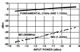
FIGURE 16. IM3 OF PIN 4 vs INPUT POWER
