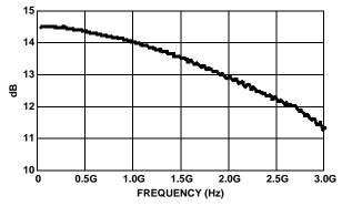
FIGURE 7. |S21| vs FREQUENCY
