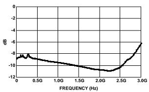
FIGURE 13. |S33| vs FREQUENCY
