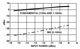
FIGURE 19. IM2 OF PIN 4 vs INPUT POWER
