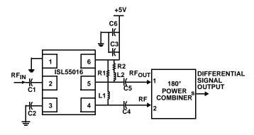
FIGURE 33. EVALUATION BOARD WITH 2-WAY 180° POWER COMBINER
