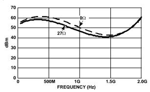
FIGURE 26. DIFFERENTIAL OIP2 vs FREQUENCY
