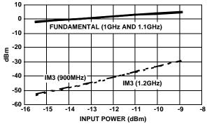
FIGURE 17. IM3 OF PIN 5 vs INPUT POWER
