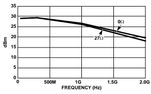
FIGURE 28. DIFFERENTIAL OIP3 vs FREQUENCY
