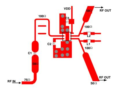
FIGURE 31. PCB LAYOUT OF MATCHING NETWORK
