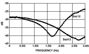
FIGURE 5. |Ssd12| AND |Ssc12| vs FREQUENCY
