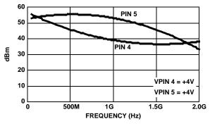
FIGURE 21. OIP2 vs FREQUENCY
