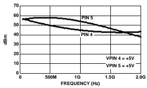
FIGURE 22. OIP2 vs FREQUENCY
