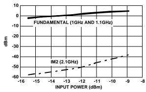
FIGURE 20. IM2 OF PIN 5 vs INPUT POWER
