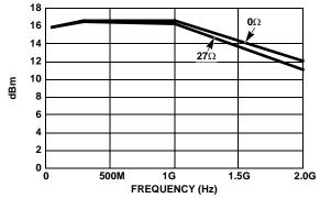
FIGURE 25. DIFFERENTIAL P1dB vs FREQUENCY
