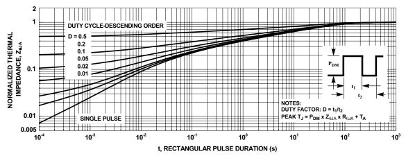
Figure 11. Transient Thermal Response Curve
