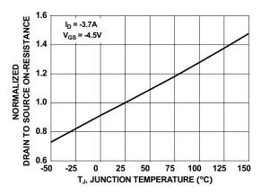
Figure 3. Normalized On-Resistance vs Junction Temperature
