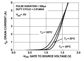
Figure 5. Transfer Characteristics
