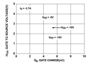
Figure 7. Gate Charge Characteristics
