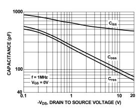
Figure 8. Capacitance Characteristics
