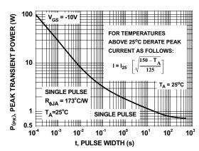
Figure 10. Single Pulse Maximum Power Dissipation
