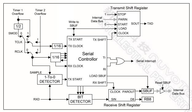
Figure 14-2 Serial Port Mode 1
