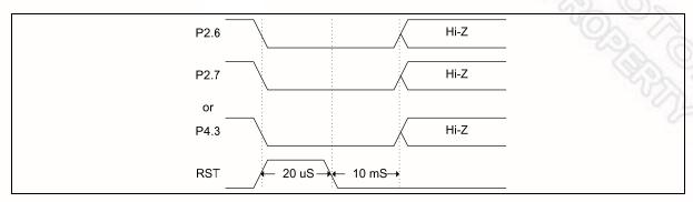
Figure 19-1 Timing of Entering Re-Boot Mode
