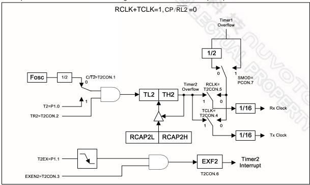
Figure 11-7 Baud Rate Generator Mode
