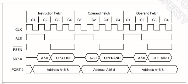
Figure 7-3 Three Cycle Instruction Timing
