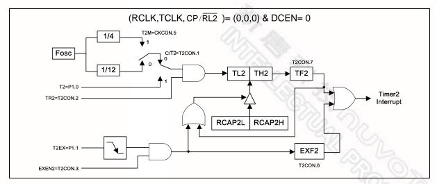
Figure 11-5 16-Bit Auto-reload Mode, Counting Up
