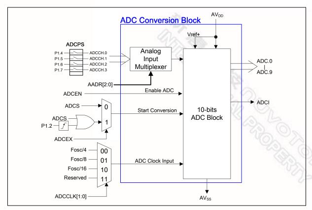
Figure 16-2 ADC Block Diagram
