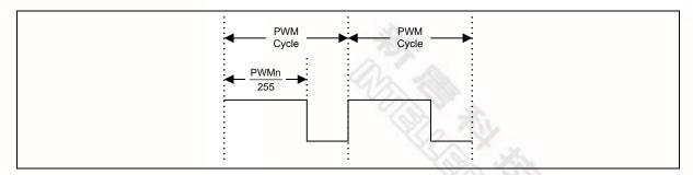
Figure 13-2 PWM Duty Ratio
