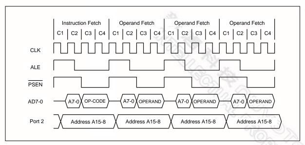
Figure 7-4 Four Cycle Instruction Timing
