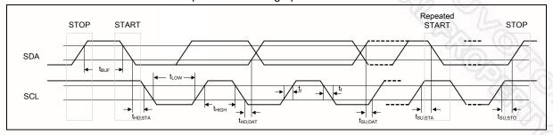
Figure 15-1 I2C Bus Timing
