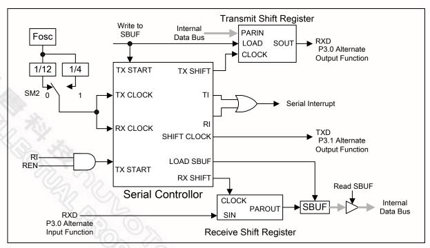
Figure 14-1 Serial Port Mode 0
