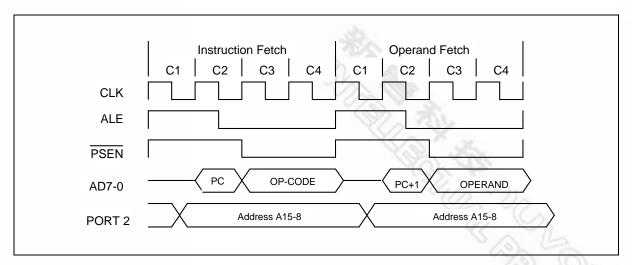
Figure 7-2 Two Cycle Instruction Timing
