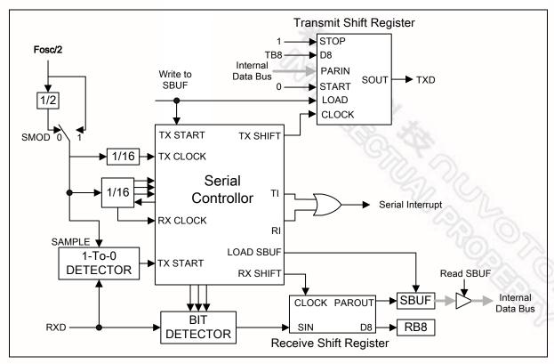
Figure 14-3 Serial Port Mode 2
