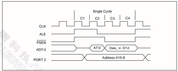
Figure 7-1 Single Cycle Instruction Timing
