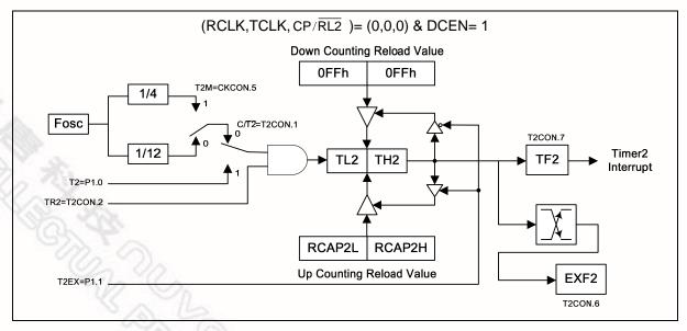
Figure 11-6 16-Bit Auto-reload Up/Down Counter
