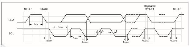
Figure 23-1 I2C Bus Timing
