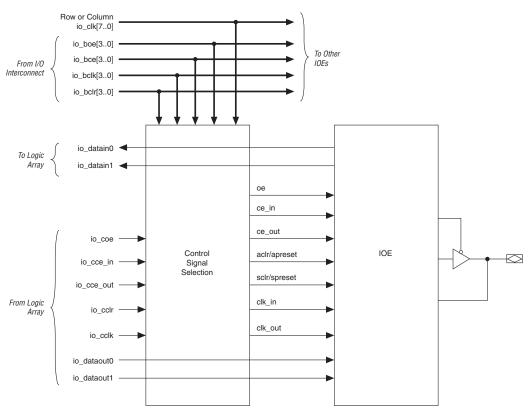
Each IOE contains its own control signal selection for the following control signals: oe, ce\_in, ce\_out, aclr/preset, sclr/preset, clk\_in, and clk\_out. Figure 2–63 illustrates the control signal selection.
