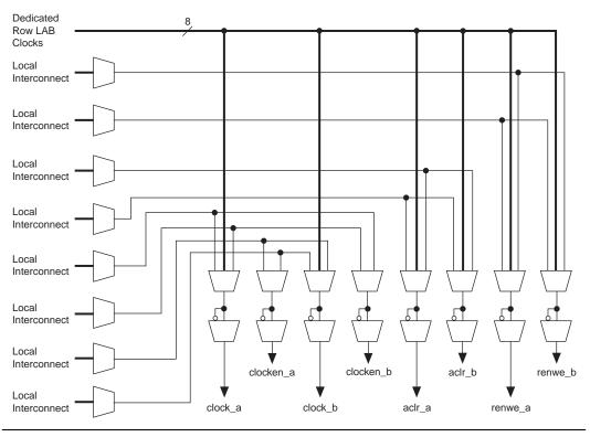
Figure 2–19. M-RAM Block Control Signals
