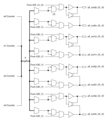
Figure 2–55. External Clock Outputs for PLLs 5 & 6
