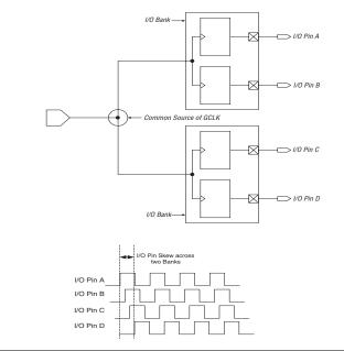
Table 4–97 defines the timing parameters used to define the timing for horizontal I/O pins (side banks 1, 2, 5, 6) and vertical I/O pins (top and bottom banks 3, 4, 7, 8). The timing parameters define the skew within an I/O bank, across two neighboring I/O banks on the same side of the device, across all horizontal I/O banks, across all vertical I/O banks, and the skew for the overall device.
