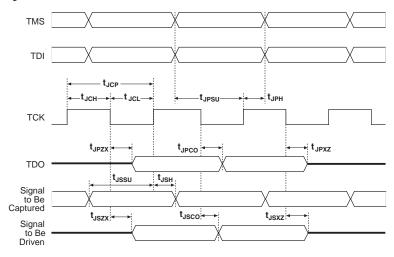
Figure 3–1. Stratix JTAG Waveforms
