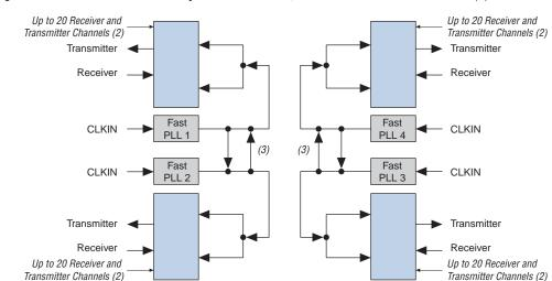
Figure 2–74. Fast PLL & Channel Layout in the EP1S10, EP1S20 or EP1S25 Devices Note (1)
