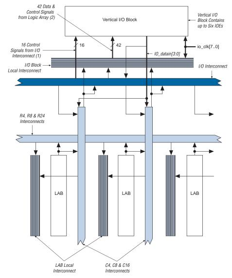
Figure 2–61. Column I/O Block Connection to the Interconnect
