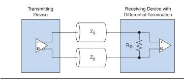
Figure 2–71. LVDS Input Differential On-Chip Termination
