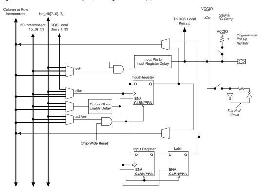
Figure 2–65. Stratix IOE in DDR Input I/O Configuration Note (1)
