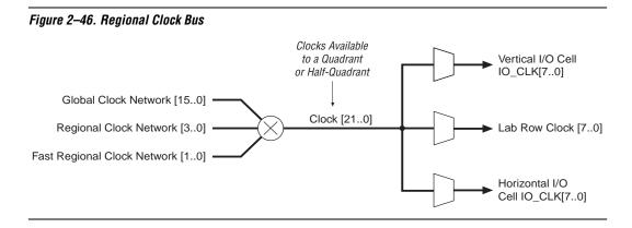
IOE clocks have horizontal and vertical block regions that are clocked by eight I/O clock signals chosen from the 22 quadrant or half-quadrant clock resources. Figures 2–47 and 2–48 show the quadrant and halfquadrant relationship to the I/O clock regions, respectively. The vertical regions (column pins) have less clock delay than the horizontal regions (row pins).
