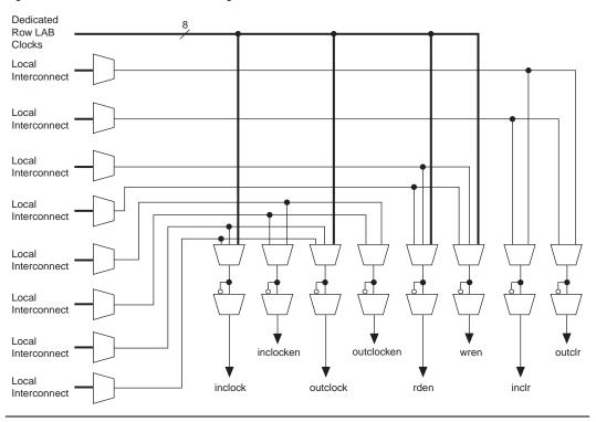
Figure 2–15. M512 RAM Block Control Signals
