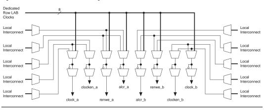
Figure 2–17. M4K RAM Block Control Signals
