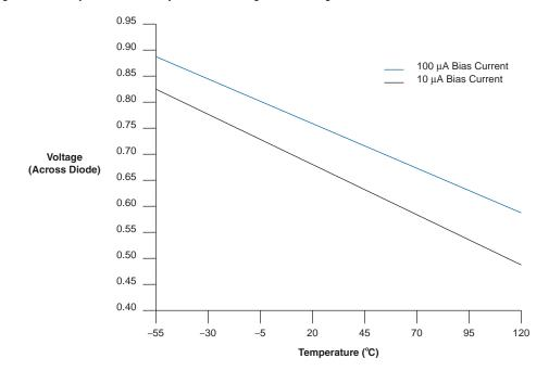
Figure 3–6. Temperature vs. Temperature-Sensing Diode Voltage
