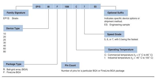
Figure 5–1. Stratix Device Packaging Ordering Information
