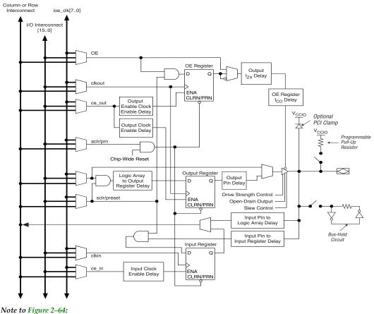
Figure 2–64. Stratix IOE in Bidirectional I/O Configuration Note (1)
