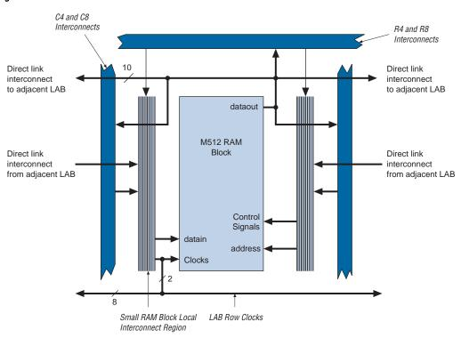
Figure 2–16. M512 RAM Block LAB Row Interface
