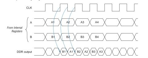
The Stratix IOE operates in bidirectional DDR mode by combining the DDR input and DDR output configurations. Stratix device I/O pins transfer data on a DDR bidirectional bus to support DDR SDRAM. The negative-edge-clocked OE register holds the OE signal inactive until the falling edge of the clock. This is done to meet DDR SDRAM timing requirements.
