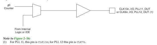
Stratix devices can drive any enhanced PLL driven through the global clock or regional clock network to any general I/O pin as an external output clock. The jitter on the output clock is not guaranteed for these cases.
