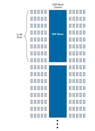
Figure 2–29. DSP Blocks Arranged in Columns
