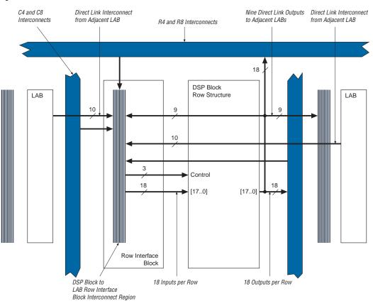
Figure 2–41. DSP Block Interface to Interconnect
