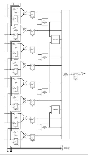
Figure 2–31. DSP Block Diagram for  $9 \times 9$ -Bit Configuration
