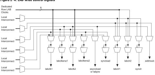
Figure 2–4. LAB-Wide Control Signals
