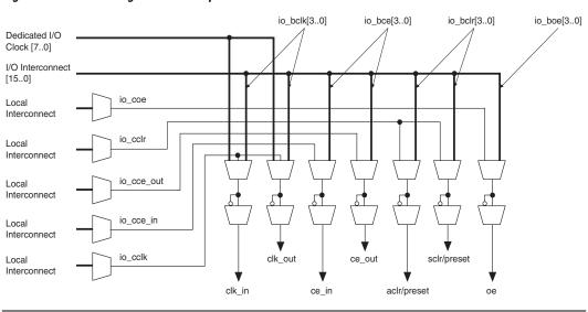
Figure 2–63. Control Signal Selection per IOE
