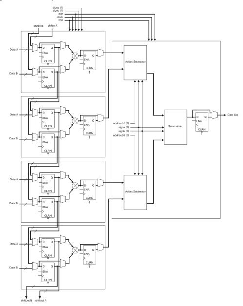
Figure 2–39. Four-Multipliers Adder Mode
