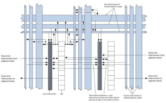
Figure 2–2. Stratix LAB Structure
