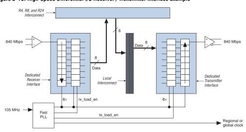
Figure 2–73. High-Speed Differential I/O Receiver / Transmitter Interface Example
