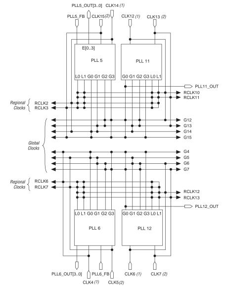
Figure 2–51. Global & Regional Clock Connections from Top Clock Pins & Enhanced PLL Outputs Note (1)
