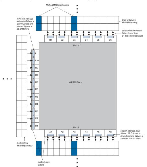
Figure 2–21. Left-Facing M-RAM to Interconnect Interface Notes (1), (2)
