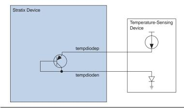
Figure 3–5. External Temperature-Sensing Diode
