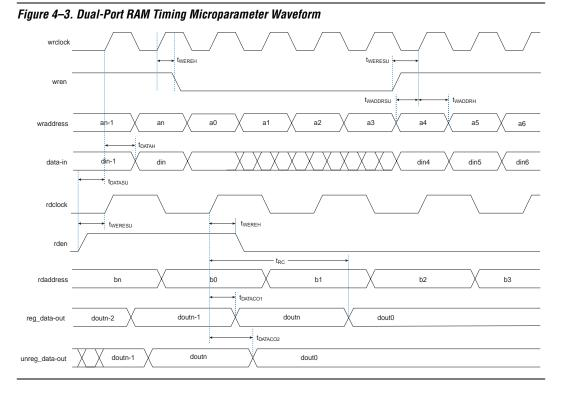
Figure 4–3 shows the TriMatrix memory waveforms for the M512, M4K, and M-RAM timing parameters shown in Tables 4–40 through 4–42.
