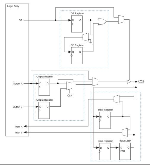
The IOEs are located in I/O blocks around the periphery of the Stratix device. There are up to four IOEs per row I/O block and six IOEs per column I/O block. The row I/O blocks drive row, column, or direct link interconnects. The column I/O blocks drive column interconnects. Figure 2–60 shows how a row I/O block connects to the logic array. Figure 2–61 shows how a column I/O block connects to the logic array.
