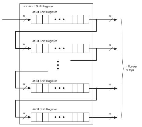
Figure 2–14. Shift Register Memory Configuration
