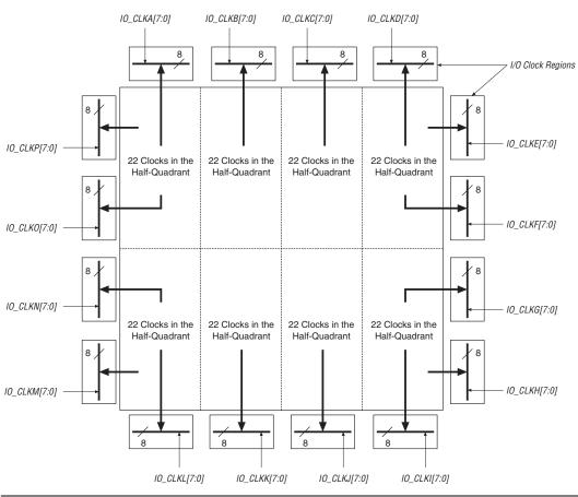
Figure 2–48. EP1S30, EP1S40, EP1S60, EP1S80 Device I/O Clock Groups
