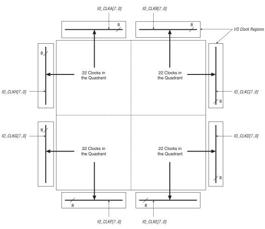
Figure 2–47. EP1S10, EP1S20 & EP1S25 Device I/O Clock Groups
