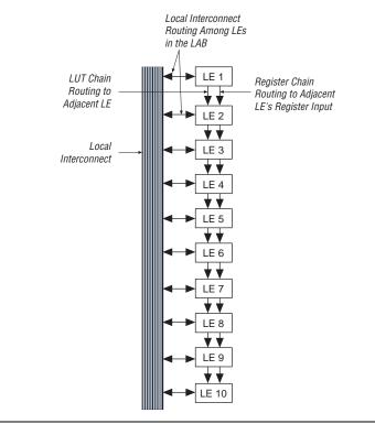
Figure 2–10. LUT Chain & Register Chain Interconnects
