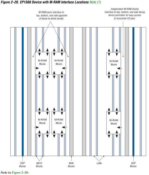
(1)Device shown is an EP1S60 device. The number and position of M-RAM blocks varies in other devices.
