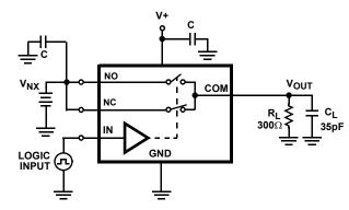
Repeat test for all switches.  $\mathsf{C}_{\mathsf{L}}$  includes fixture and stray capacitance.
