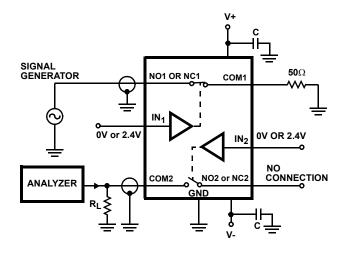
FIGURE 6. CROSSTALK TEST CIRCUIT
