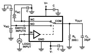
Repeat test for all switches.  $\ensuremath{\mathsf{C}}_L$  includes fixture and stray capacitance.
