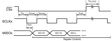
Figure 29: SPI Interface Timings Output
