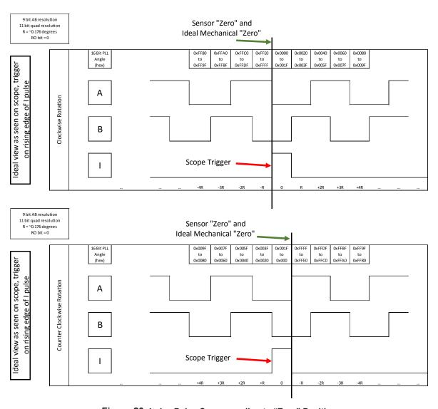
Figure 20: Index Pulse Corresponding to "Zero" Position
