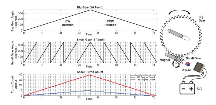
Figure 25: Example of a Turns Counting Application
