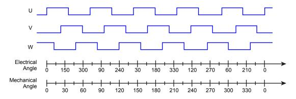
Figure 23: U, V, W Outputs for Five Pole-Pair BLDC Motor
