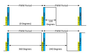
Figure 15: Pulse-Width Modulation (PWM) Examples
