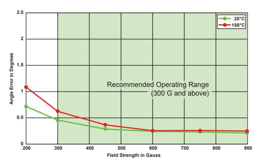
Figure 48: Angle Error over Field Strength
