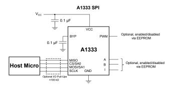
Typical A1333 configuration using SPI interface.
