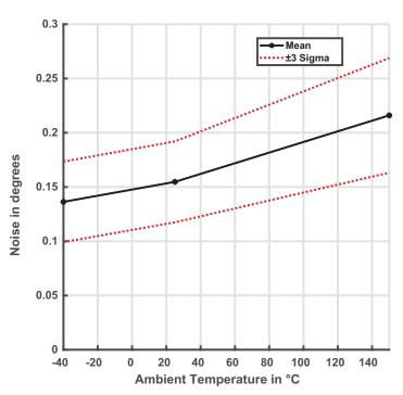
Figure 7: Noise Performance over Temperature (3 Sigma, 300 G)
