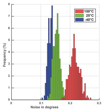
Figure 9: Noise Distribution over Temperature (3 Sigma, 300 G)
