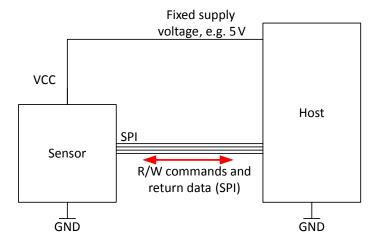
Figure 27: SPI Interface Programming Setup
