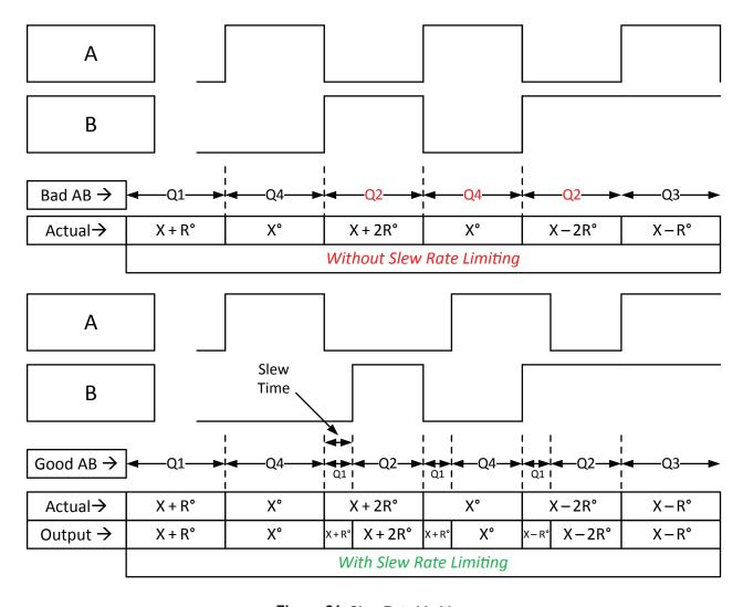
Figure 21: Slew Rate Limiting
