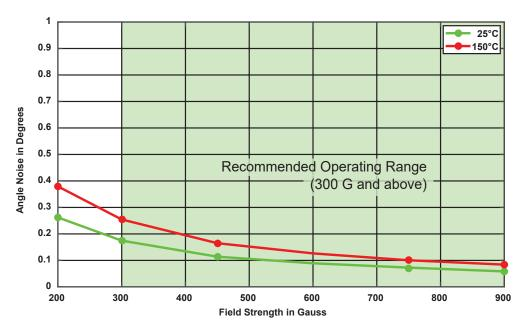
Figure 49: Noise (3 Sigma) over Field Strength
