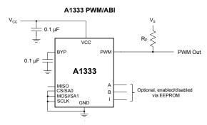
Typical A1333 configuration using PWM output. Digital reads/writes requests transmitted via Manchester encoding on the  $V_{\rm CC}$  line. SA0/SA1 brought to BYP or GND to configure Manchester address.
