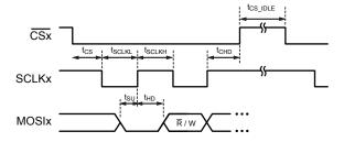
Figure 28: SPI Interface Timings Input
