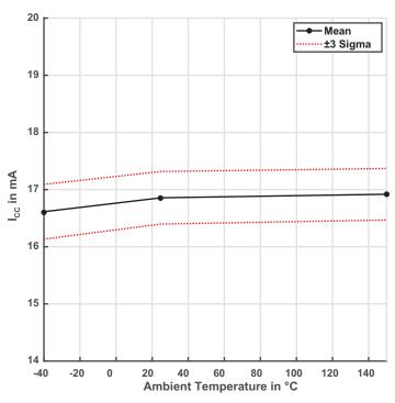
Figure 8:  $I_{CC}$  over Temperature ( $V_{CC}$  = 16.0 V)
