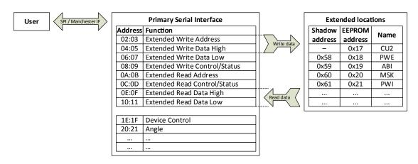
Figure 26: Serial Registers allow access to extended memory (EEPROM and Shadow)
