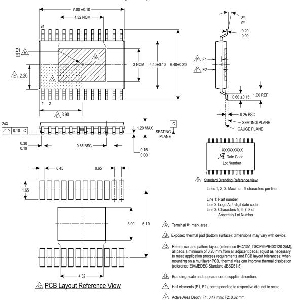
Figure 50: Package LP, 24-Pin TSSOP with Exposed Thermal Pad
