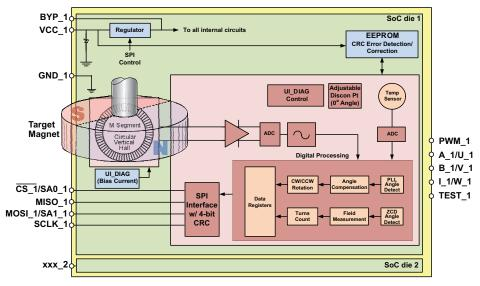
Figure 1: A1333 Magnetic Circuit and IC Diagram
