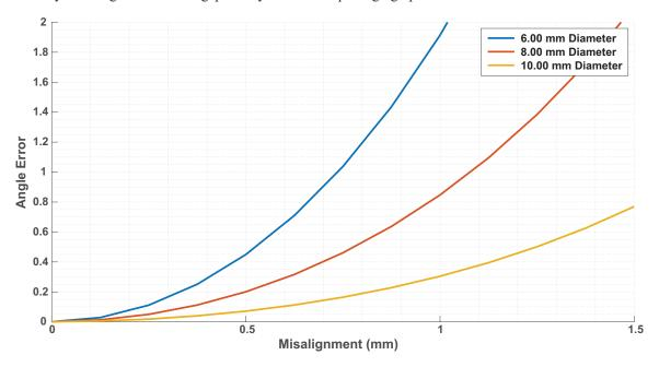
Figure 46: Simulated Error versus Eccentricity for different size magnet diameters, at 2.0 mm air gap
