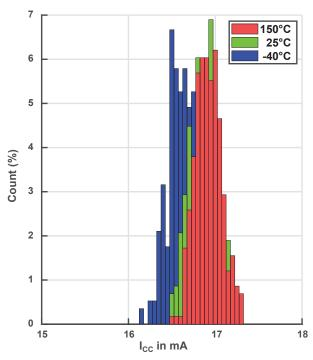
Figure 10:  $I_{CC}$  Distribution over Temperature  $(V_{CC} = 16.0 \text{ V})$
