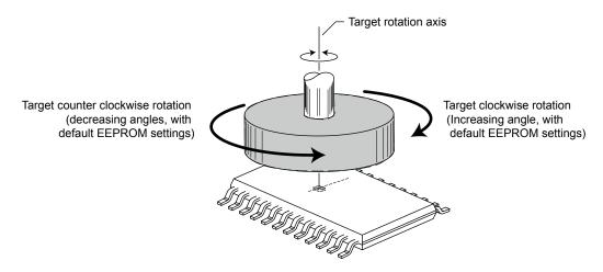
Figure 47: Rotation Direction Definition
