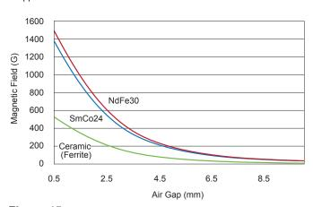
Figure 45: Magnetic Field versus Air Gap for a magnet 6 mm in diameter and 2.5 mm thick.
