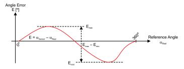
Figure 52: Angle Error Definition
