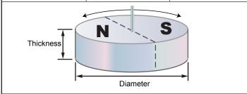
\* A sintered Neodymium magnet with 10 mm (or greater) diameter and 2.5 mm thickness is the recommended magnet for redundant applications.
