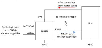
Figure 35: Manchester Interface Programming Setup
