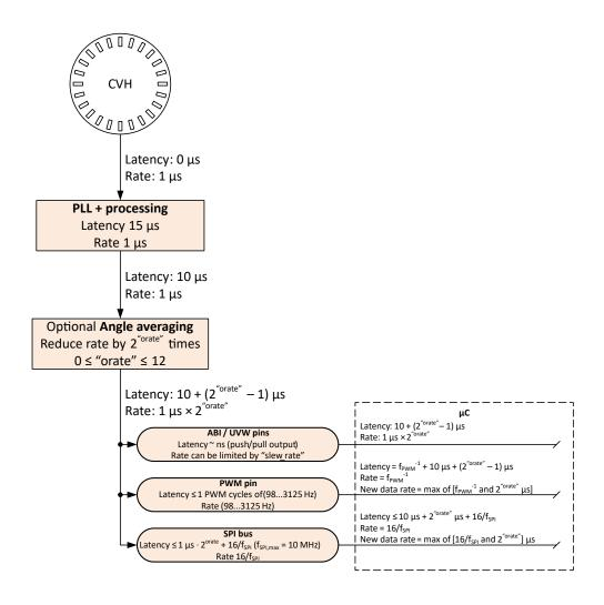
Figure 12: Update Rate and Signal Delay
