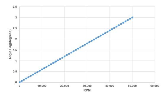
Figure 11: Angle Lag vs. RPM (10 µs Response Time)
