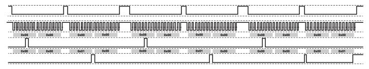
If an access violation occurs (address not unlocked), the transaction will be terminated and the corresponding "rdn" or "wdn" bit set, and the "xee" warning bit will assert. The "xee" bit in the "err" register will also set if the EEPROM write aborts.
