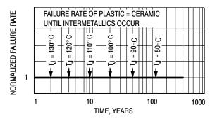
Figure 3. Failure Rate vs. Time Junction Temperature
